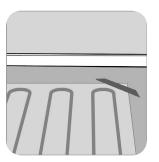
You may also need to remove a small section of underlayment from under the mat at the point where the power supply cord enters the mat, to prevent an unsightly lump on the Laminate or carpet surface and excessive wear on that part of the mat.
