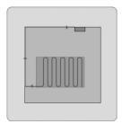
Once the underlayment/insulation has been fitted in the normal manner, remove your Warmup® Foil mat from the packaging box, unroll it completely and place it in the required position on top of the underlayment/insulation. Make sure that Warmup Foil heating mats are installed with the correct orientation. The side marked "THIS SIDE UP" is facing upwards.
